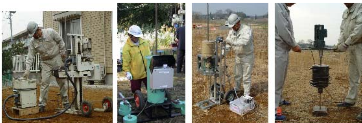
Photograph 1 Examples of automatic and electric Swedish sounding machines used in Japan
