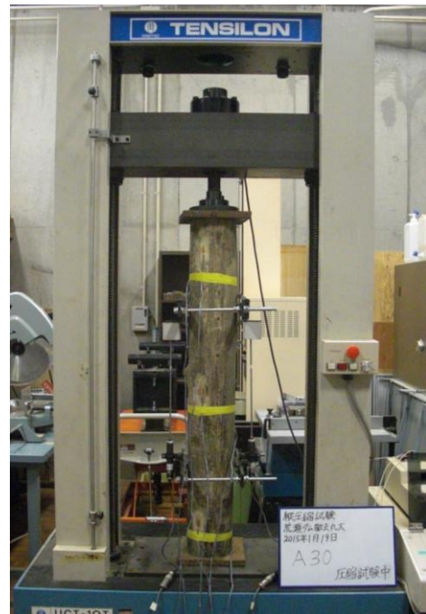
Photo 6: Longitudinal Young's modulus testing
