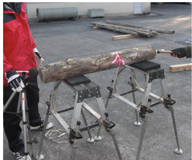
Photo 7: Longitudinal vibration testing.
